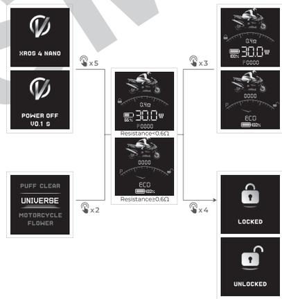
The diagram shows the sequence of screen displays when the fire button is pressed multiple times: 1. XROS 4 NANO (x5), 2. POWER OFF (x3), 3. Resistance: 0.6Ω (x3), 4. PUFF CLEAR (x2), 5. UNIVERSE MOTORCYCLE FLOHER (x2), 6. LOCKED (x4), 7. UNLOCKED (x4).
